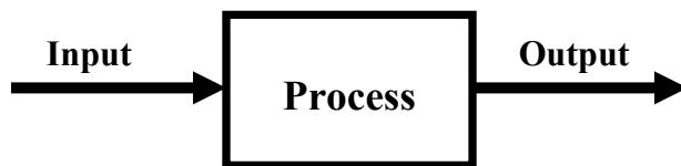
A machine is a process or, rather, a processor. The machine takes input and does something to it. The machine gives output that is more useful to the system users (in a particular context) than was the original input. The output of the machine is "*the good thing that we want it to do*" – ie the "function" or purpose of the machine such as lifting a heavy load of bricks.
