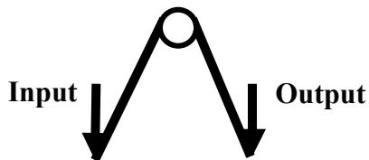
Our original ideal machine, the lever, had one long horizontal member – a beam -- that did not deform when in use. In other words, the lever's beam did not bend appreciably under loading. Bending is a combination of compression and tension. In the three 'kinked beam' models above, the beam is kinked around the fulcrum but it is still a continuous and rigid beam nonetheless.
