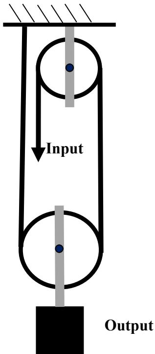
You may be tempted to say that the object is only acted upon by two forces, as in the previous model – gravity pulling down and the bracket pulling it up. However, you can state your assumption that the object and lower pulley are connected to each other such that they become another object --- another free body. And it could very well be that the weight of the lower pulley / bracket is very small compared to the weight of the object load.
