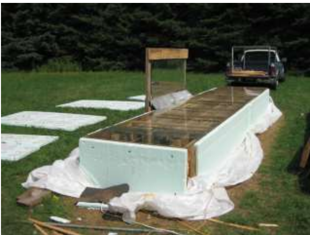
Very “quick-and-dirty” solar powered lumber drying kiln in Pickering (with electric-assist to maintain temperature overnight.)
