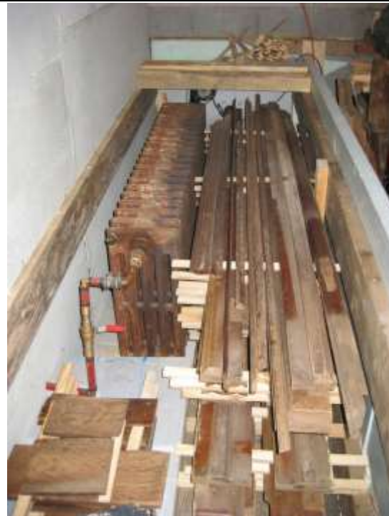
Wood-fired-hydronic lumber-drying kiln. Heat-treating oak trim from a 1917 Scarborough farmhouse.
