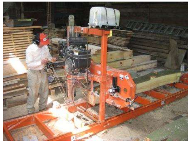
Portable sawmill in Pickering, 2010 – gasoline engine-driven.
